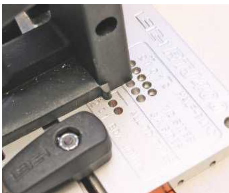
▲ This black rod slides into a channel on the jig
